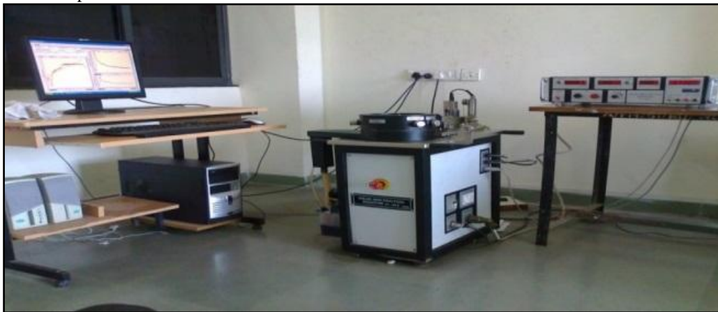
Fig.3. Photograph of Experimental Set up Of Pin-On-Disc Tribometer
